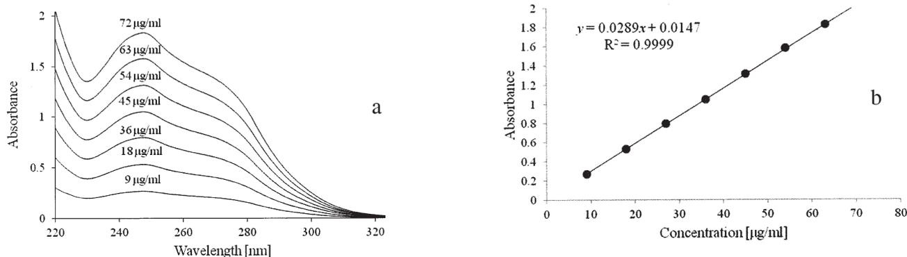
Fig. 5. a) UV absorption spectra of ZOF in distilled water, with concentrations ranging between 9 and 72 µg/mL; b) the calibration curve of ZOF in distilled water.
