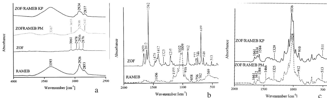
Fig. 4. ATR-FTIR spectra of: a) RAMEB, ZOF, ZOF/RAMEB physical mixture and ZOF/RAMEB kneaded product in 4000-2500  $\text{cm}^{-1}$  spectral region; b) ZOF and RAMEB in 2000-500  $\text{cm}^{-1}$  spectral region; c) ZOF/RAMEB PM and ZOF/RAMEB KP in 2000-500  $\text{cm}^{-1}$  spectral region
