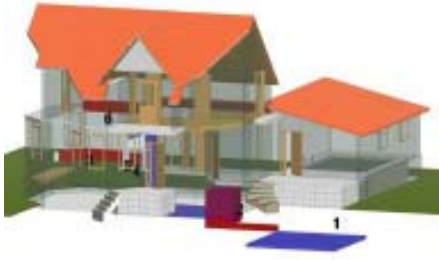
Fig.2. Family house equipped with experimental filtration system; Isometric diagram of filtration and ventilation
