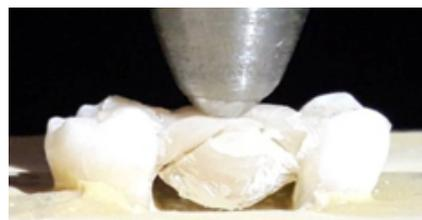
Fig. 3. Fracture pattern for parallel design of the fibres
