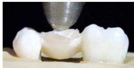
Fig. 4. Fracture pattern for adjacent design of the fibres
