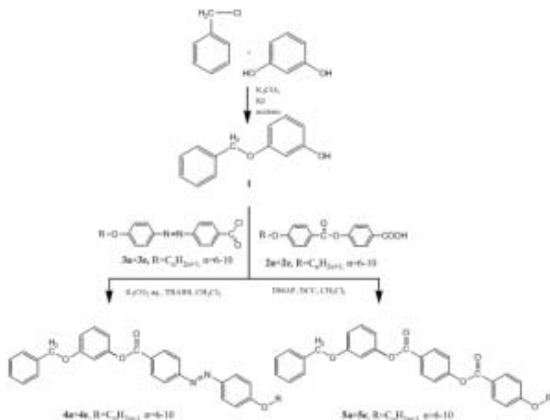
Scheme 1. Synthesis of bent-core liquid crystals compounds compounds of 4a ÷ 4e series present liquid crystalline behaviour only on the cooling cycle. The first compound with six atoms in the flexible chain shows an unidentified texture in the form of long leaves which grow from isotropic
