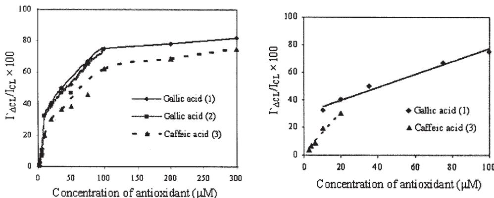
Fig. 3. Calibration curves  $(I'_{\text{ACL}}/I_{\text{CL}} \times 100)$  as a function of gallic acid (curves 1 and 2) and respectively caffeic acid (curve 3) concentrations ( $\mu\text{M}$ ). A. calibration curves; B. linearity domain. Working procedure as above. Calibration curves for gallic acid were drawn in the same conditions but at 24 h time interval
