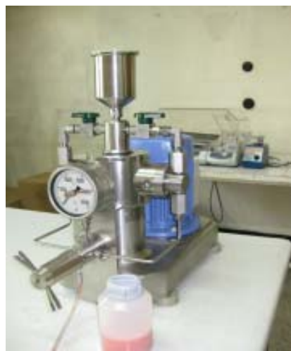
Fig. 1 Experimental setup High pressure homogeniser - Ika Werke
