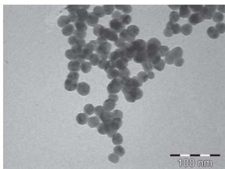
Fig. 3. Typical TEM image for AuNps 22-24nm
