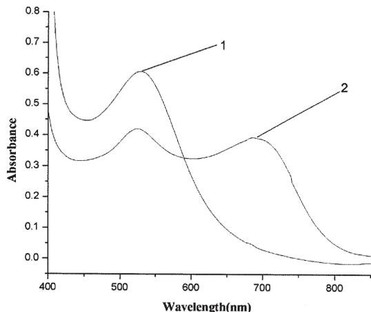
Fig. 1 UV-Vis spectra of gold nanoparticles (AuNps): 1- AuNps for size 2-5nm; 2 – AuNps for size 22-24nm
