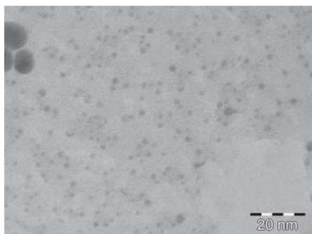
Fig. 2. Typical TEM image for AuNps 2-5nm.
