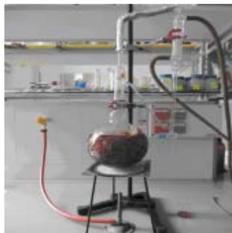
Fig. 2 The photograph of the Clevenger hydrodistillation installation
