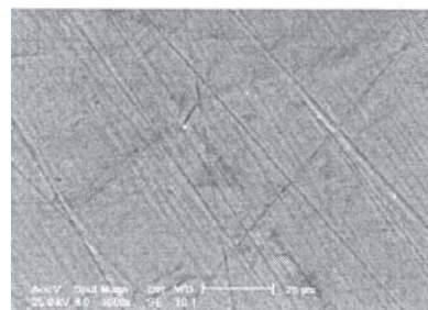
Fig. 1. SEM image of polished CoCrMo alloys
