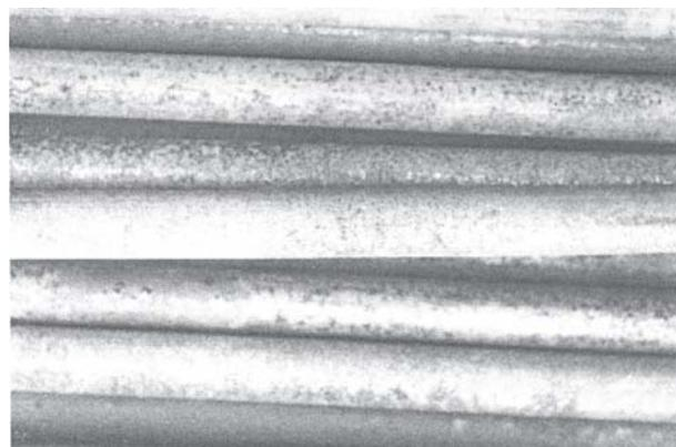
Fig. 5. Local corrosion presented as points and spots and iron oxides deposit on carbon steel tubes of the heat exchanger (external surface) - macroscopic picture
