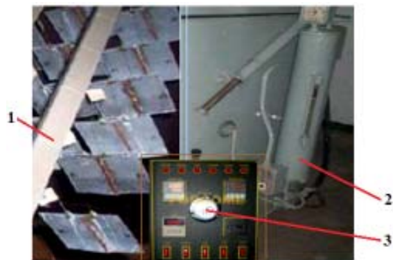
Fig. 2. Installation for testing specimens in salt fog chamber (solution 5% NaCl) ; 1 – the chamber with the mounting racks, 2 – general view of the system with the pressure cylinder for salt solution, 3 – the control panel (SC METAV-CD SA Bucharest)
