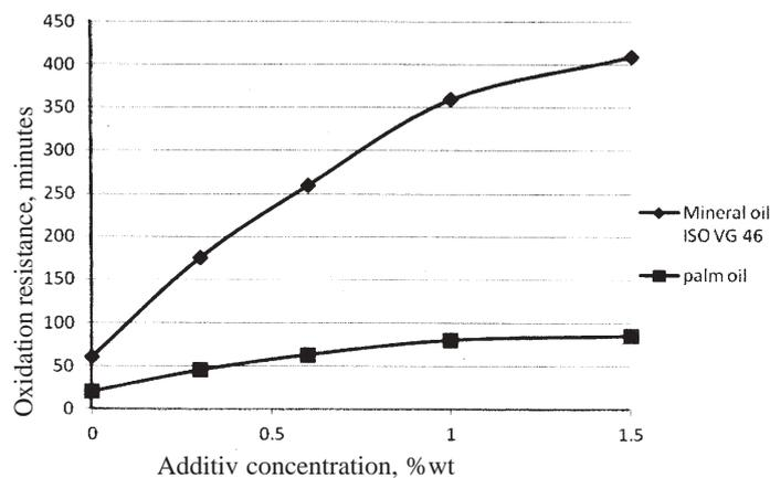
Fig. 4 Comparison between ISO VG 46 mineral oil and palm oil
