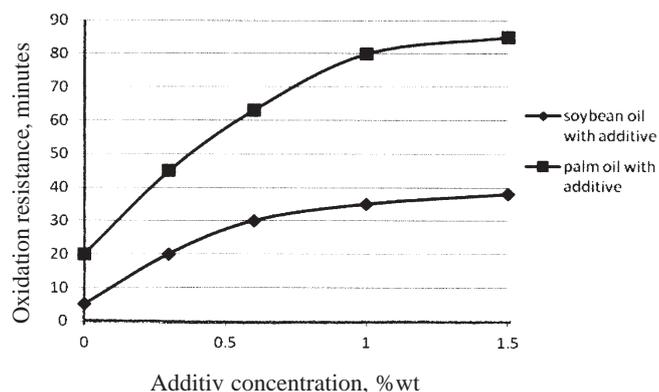
Fig. 1 Oxidation resistance of vegetable oils mixed with additive
