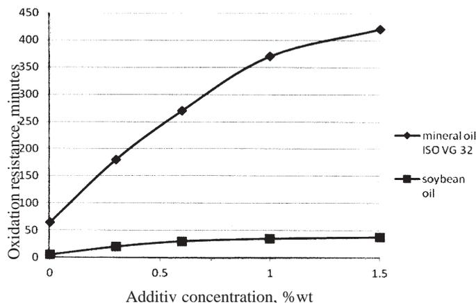
Fig. 2 Oxidation resistance of mineral oils mixed with additive
