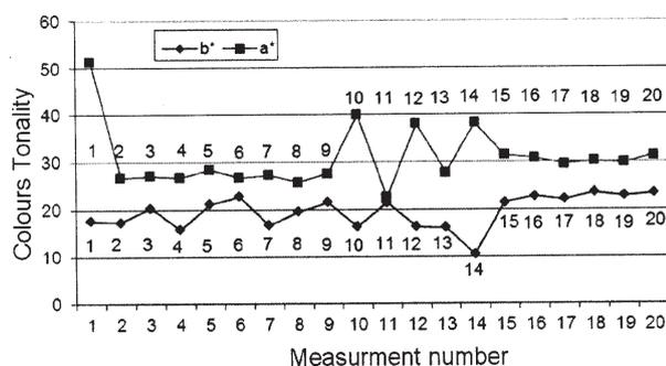
Fig. 5. The red degree dynamic for activated samples
