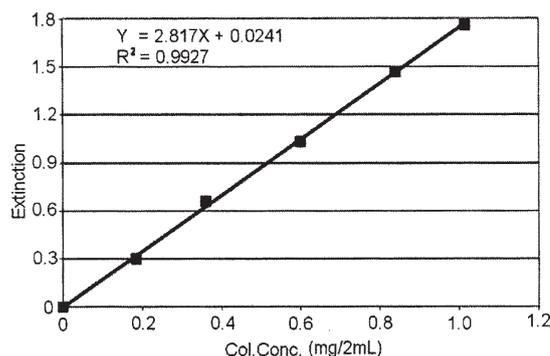
Fig. 2. The calibrator curve obtained at the spectrophotometric dosage in UV of carthamin
