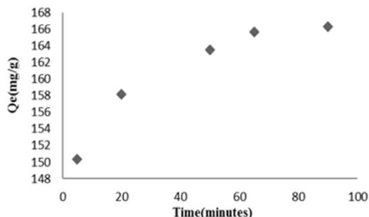
Fig. 1. Effect of the contact time on the GNB sorption onto strongly basic anion exchange resin Amberlite IRA 400
