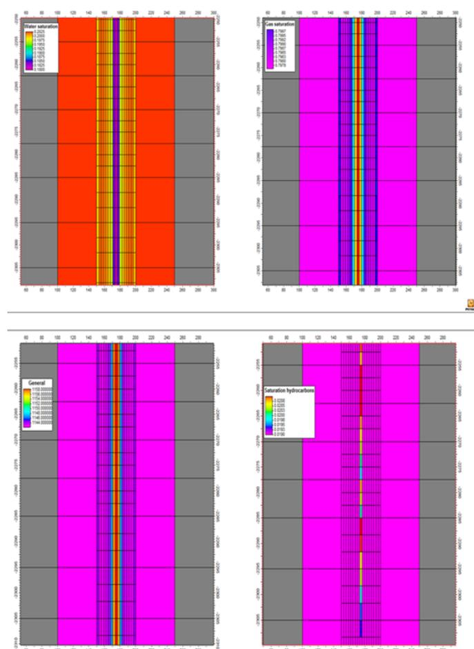
Fig. 5. Fluid (above) & Solid Saturations (below, Right) Profile and Water Density (below, Left)
