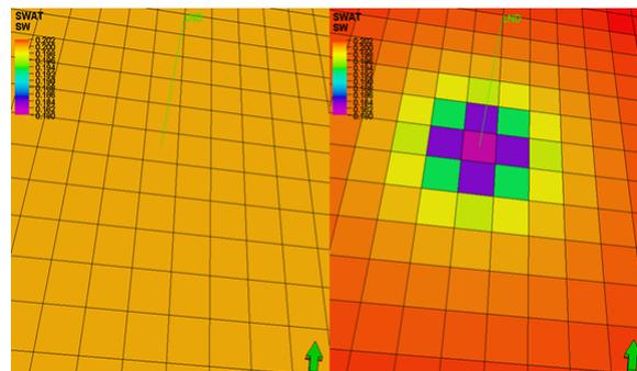
Fig.4. Water Saturation Profile at first (left) and last (right) time step - view from above
