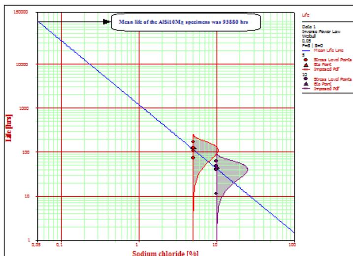
Fig. 5. The determination of the mean life of the specimens from aluminium alloy (AlSi10Mg) manufactured by SLM technology in normal use conditions
