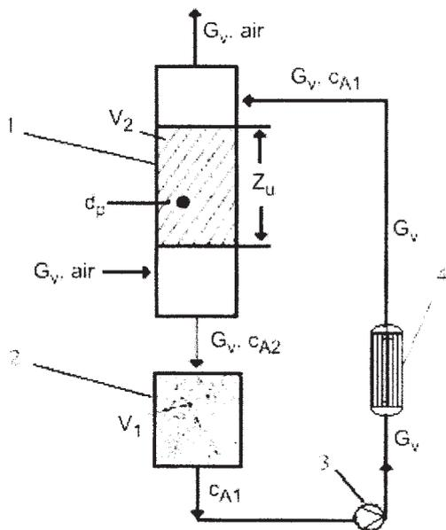
Fig. 1. Laboratory fermentation experimental set-up 1-fixed bed reactor, 2-recycling vessel, 3-recycling pump, 4- heat exchanger
