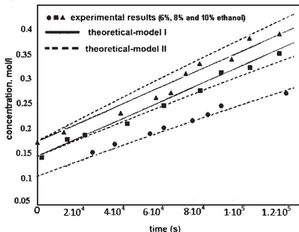
Fig. 2. Experimental and calculated acetic acid concentration vs. time for different initial ethanol concentrations at  $L_v=2.083 \cdot 10^{-6}$  m<sup>3</sup>s<sup>-1</sup> and  $G_v=9.72 \cdot 10^{-5}$  Nm<sup>3</sup> s<sup>-1</sup>
