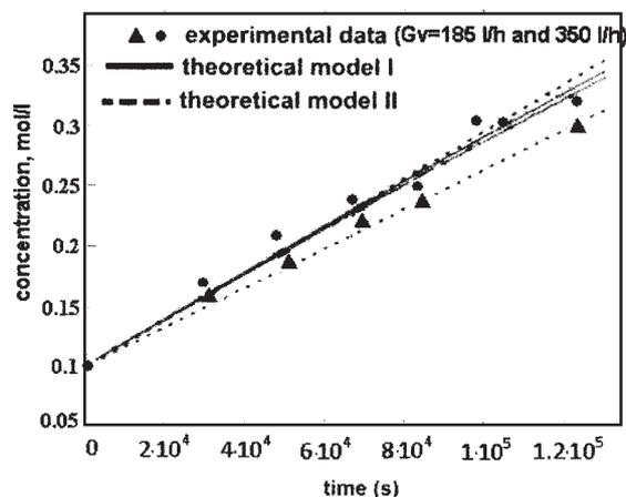
Fig. 3. Experimental and calculated acetic acid concentration vs. time for different air flow rates, at  $L_v=2.083 \cdot 10^{-6}$  m<sup>3</sup>s<sup>-1</sup>, and initial ethanol concentration  $c_{E,0}=10\%$  (mass percent)
