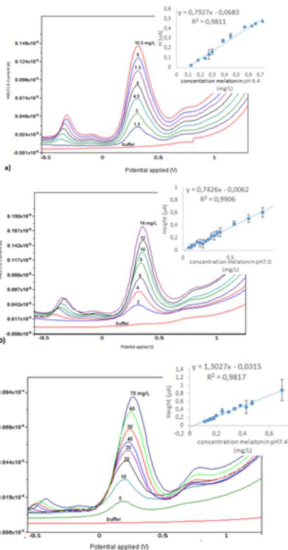
Fig. 4. DPV's measurements of melatonin solutions for pH 6.4 (a), 7.0 (b), and 7.4 (c), using DRP-150 sensor
