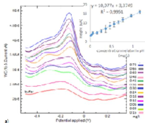
Fig. 7. DPV's peaks for different concentration of melatonin, for pH 6.4 (a) using DRP110GPH sensor
