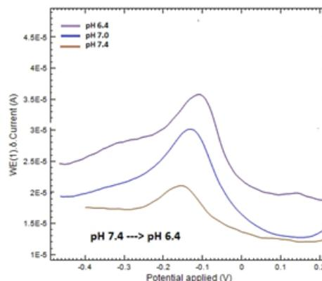
Fig. 10. Movement of peaks of DPV measurements with DRP-110GPH (for 0.66 mg/L of ML), depending on pH
