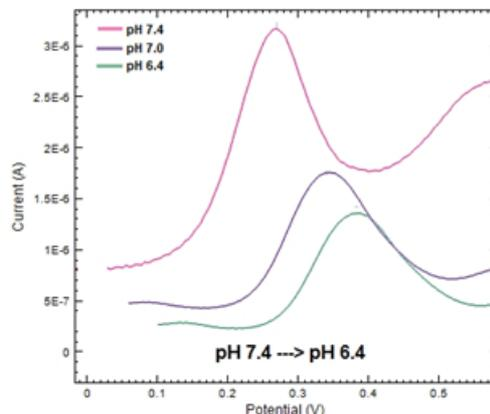
Fig. 6. Movement of 10mg/L of ML peaks depending on the pH
