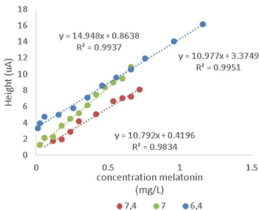
Fig. 8. Calibration lines for melatonin detection, for pH 6.4, 7.0, and 7.4
