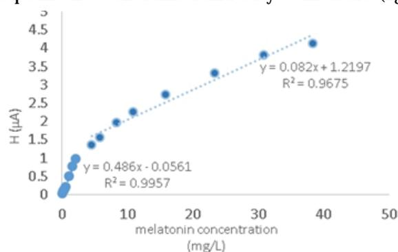
Fig. 2. Calibration curve with two liner domains, where slopes change depending on the concentration of melatonin (in range from 0.125 mg/L to 38 mg/L of ML)
