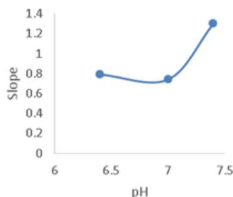
Fig. 5. Correlation between the slope of calibration lines and pH, for DVP detection of melatonin using DRP-150 sensor
