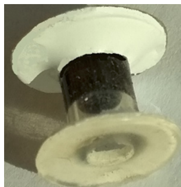
Fig. 5. Prototype of the implant with silver nano composite
